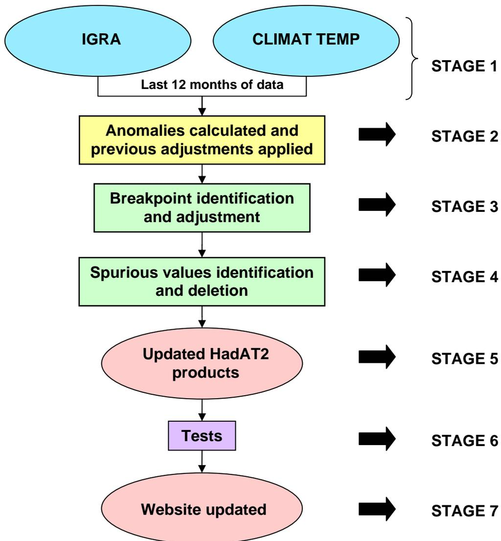
Figure 1: Schematic of the HadAT2 monthly update process
